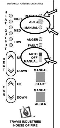
**NOTE**: if using a modulating remote, this light will come on to indicate the remote is controlling the heater.
